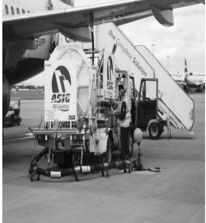
FIG. Mobile aircraft fuel dispenser for fueling from apron hydrant system.
