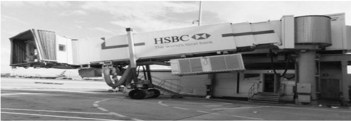
Fig. Fixed ground cooling unit attached to an air bridge.
